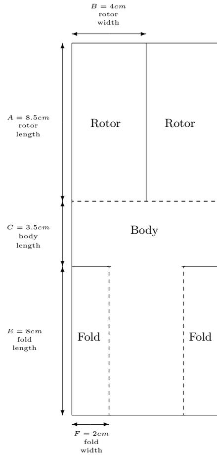
Figure 1: An example of an initial helicopter pattern
