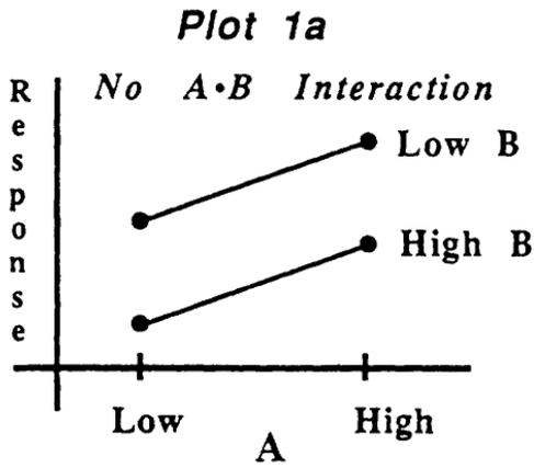
Simple, linear, additive model is sufficient.
