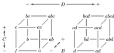
[+] Figure 3. A  $2^4$  factorial design consists of four factors, each taking two levels (+1, -1), represented here with a letter for +1 and without a letter for 1. For example, point *abd* in the figure corresponds to factors *A*, *B*, and *D* set to high level +1 and *C* to low level -1.
