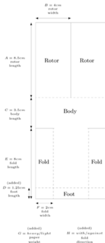
[+] Figure 1. Initial helicopter pattern. Cut along the solid lines and fold along the dotted lines. The foot fold, D , paper weight, G , and fold direction, H , were not included
